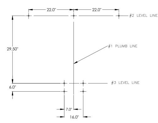
LAYOUT THE MOUNTING HOLE PATTERN AS SHOWN ABOVE. HOLES SIZED FOR 3/4" DIAMETER HARDWARE.
