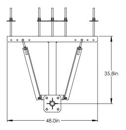
MOUNT IS SHOWN WITH THE THRU-WALL MOUNTING KIT. COMES STANDARD WITH THE WL2-36 WALL MOUNT.
