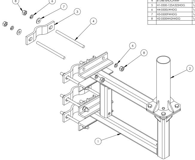
MOUNT WILL CLAMP TO 1.90"OD -3.50"OD TOWER LEG TOWER LEG NOT SHOWN
