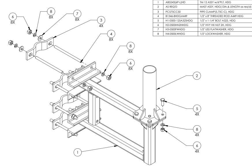
MOUNT WILL CLAMP TO 2.88"OD -4.50"OD TOWER LEG TOWER LEG NOT SHOWN
