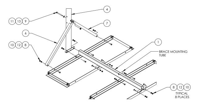
ATTACH THE SUPPORT TUBE ASS'Y(#1) TO THE BALLAST TRAYS, AS SHOWN ABOVE, USING (2) 3/8"x1" BOLTS, NUTS AND LOCK-WASHERS AT EACH ANGLE. NOTE, THE MOUNTING ANGLES FIT ON THE INSIDE OF THE 4" BALLAST TRAYS. THE MAST (#4) IS ATTACHED AT THE END OF THE MOUNT AWAY FROM THE BRACE MOUNTING TUBE.
