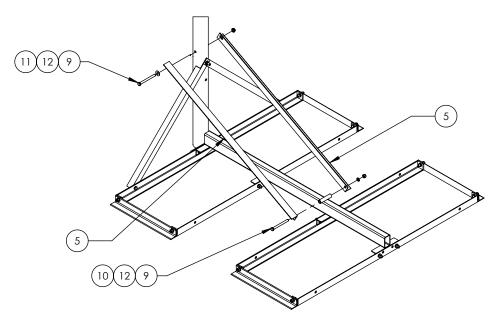
FASTEN THE TWO REAR BRACES (#5) TO THE MAST USING A 3/8"x4" FULL-THREAD BOLT, FLATWASHER AND WHIZ-LOCK NUT. NOTE: THE SLOTTED HOLE OF EACH REAR BRACE ATTACHES AT THE MAST. THE OTHER END OF EACH BRACE ATTACHES TO THE REAR BRACE MOUNTING TUBE USING A 3/8"x4" FULL-THREAD BOLT, LOCKWASHER AND NUT.
